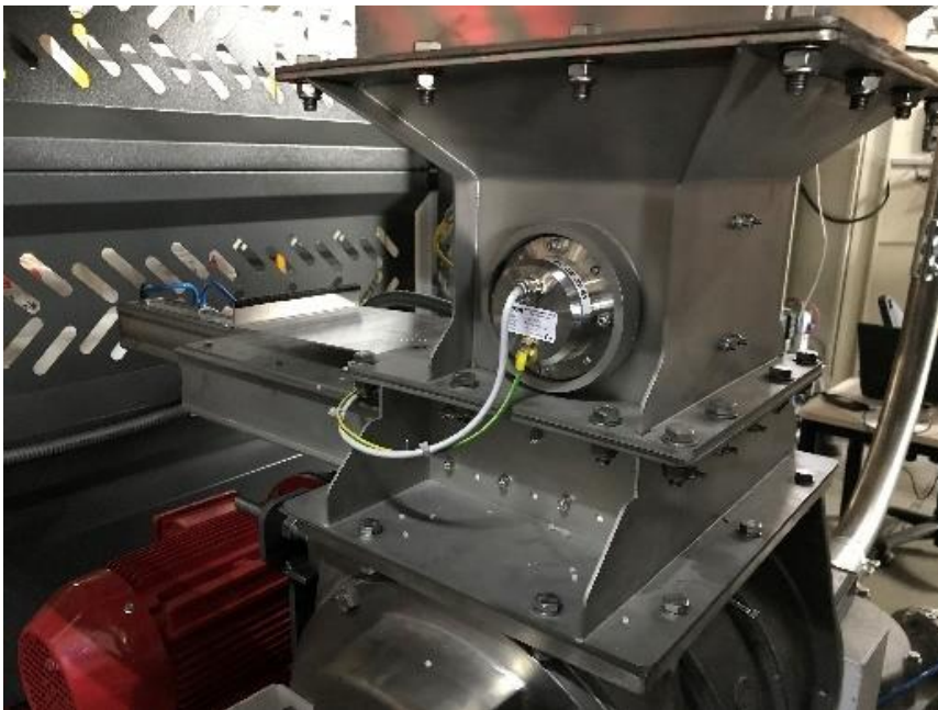
Measuring the product moisture of plastic granulate in the hopper
