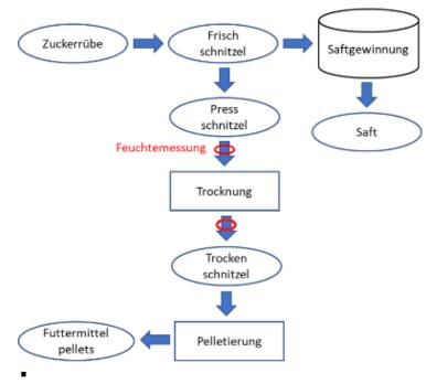
Process diagram of the sugar factory and Typical installation location for inline moisture measurement
